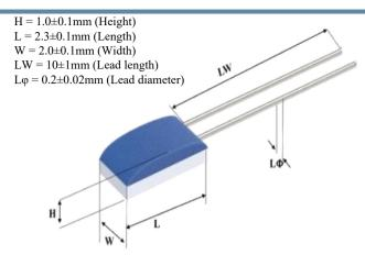
\*The nominal resistance measurement point is 8mm away from the component body
